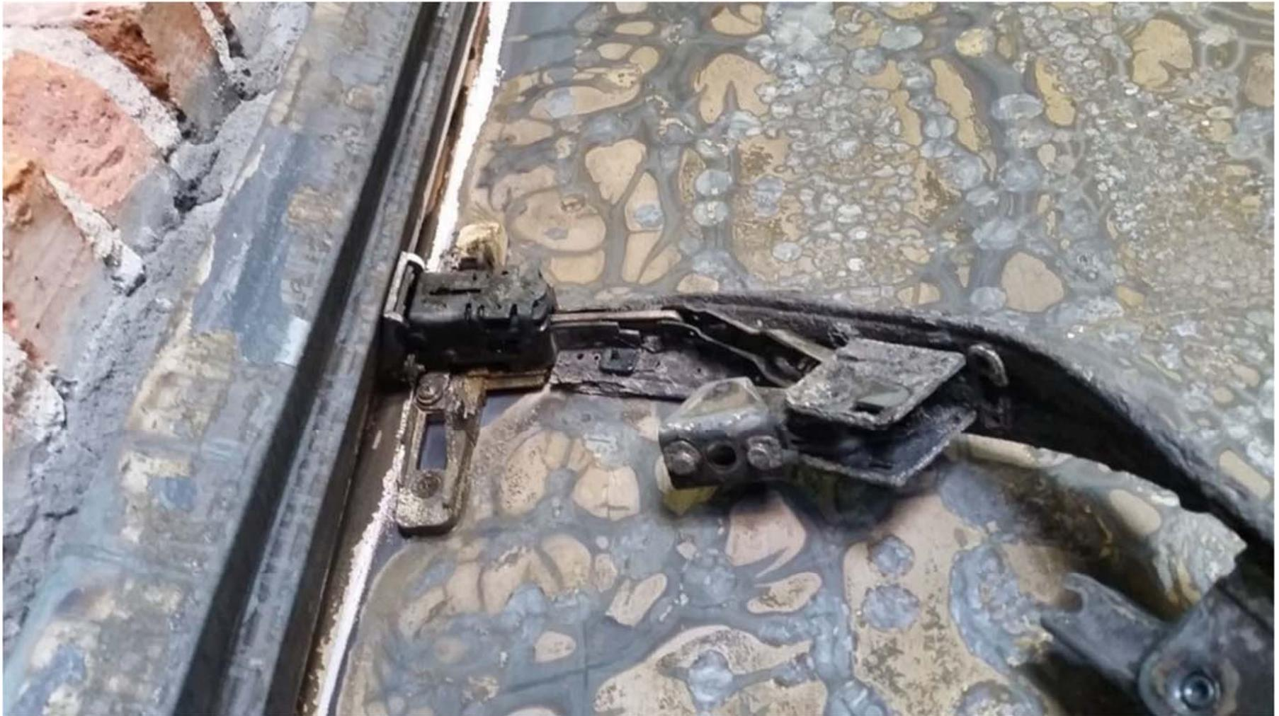
During a fire test, and potentially during a fire, the operable hardware on the door melts away and/or is deactivated by fusible material inside of the product. The latching portion remains, as the door is required to be latched for the entire duration of the test – including the hose-stream portion. But the parts normally used to retract the latch – the lever, touchpad, crossbar, etc. – no longer function in that capacity.
