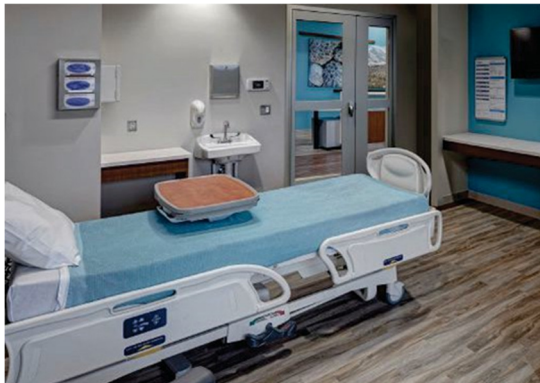
In health care occupancies, corridor doors leading to patient rooms are not required by current model codes to be fire door assemblies, but the model codes include specific requirements, including positive latching hardware on all door leaves. Allegion Photo
