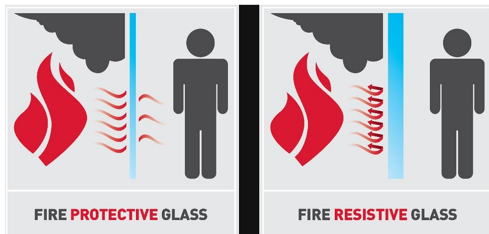
Fire-protection-rated glass stops the spread of smoke and fire while fire-resistance-rated glass blocks smoke fire, radiant and conductive heat. Credit: Courtesy of TGP
