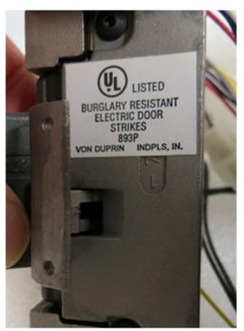
If you connect the dots, it seems obvious that a fail safe electric strike won't meet the latching requirements, and a fail secure strike won't meet the reentry requirements, so electric strikes can not be used on stairwell doors that require reentry. On other fire-rated doors that are not required to unlock upon power failure, a fail secure electric strike may be used.
