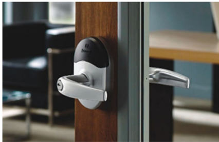
This electrified lockset incorporates a credential reader on the access side, but the inside lever always allows free egress. This is not a special locking arrangement.
